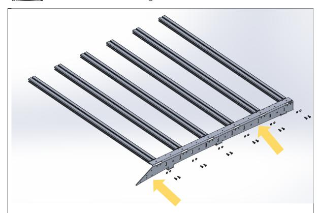
2. Fit the side rail to the extrusion,
