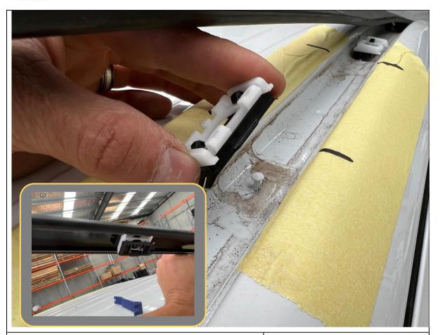
27. Once trim is removed, remove any remaining retaining clips from the mushroom studs in the roof ditch and re-fit them to the corresponding positions on the rubber ditch finisher trim.
